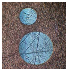
Holes cut by laser in tungsten (0.5 and 0.3 mm diameters)
